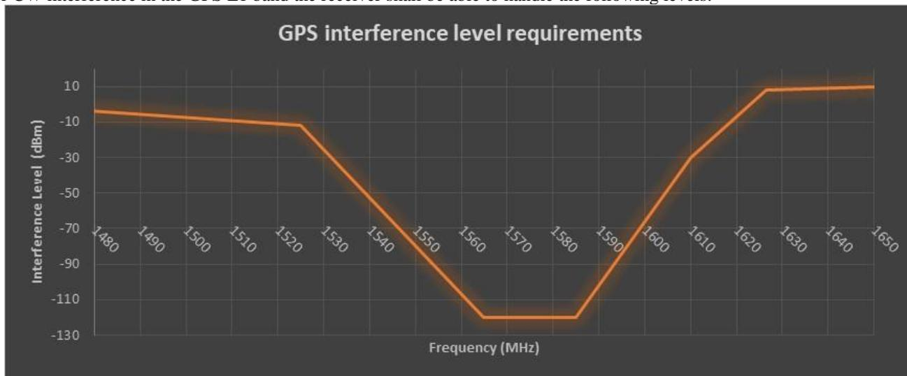
**CW interference levels for GPS (L1)**
