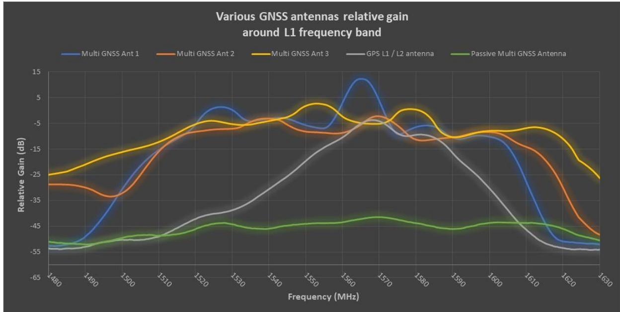
**Various multi GNSS antennas frequency response around L1 frequency band**
