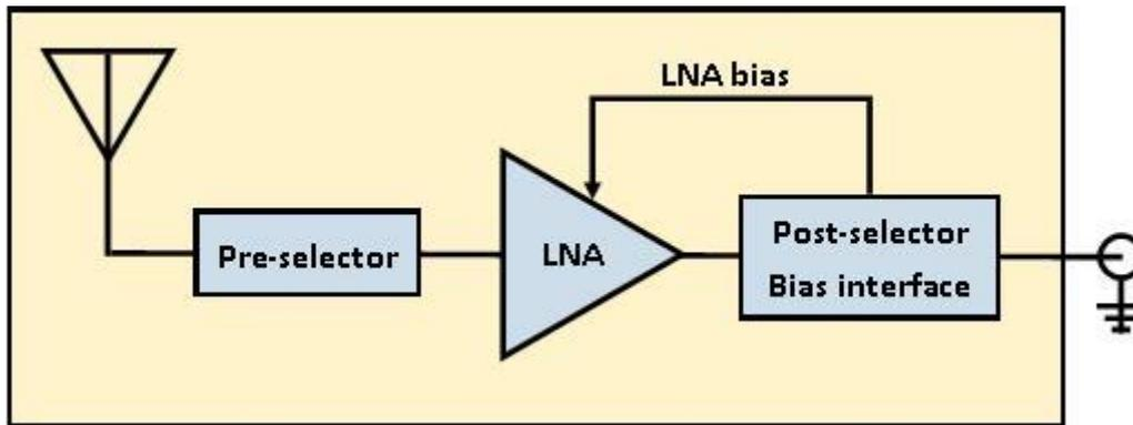
**Block Diagram for active GNSS antenna**
