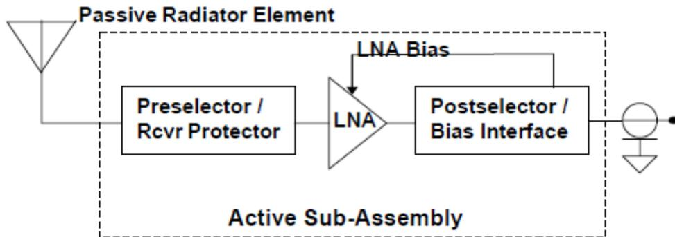
**Figure 1: Typical Block diagram of an active GNSS antenna**
