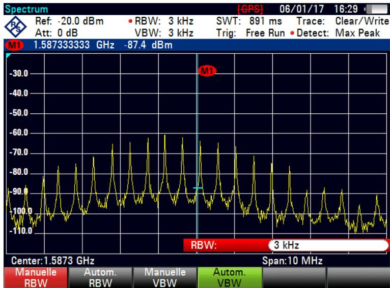
Figure 9: Screen shot of the free floating oscillator signal
