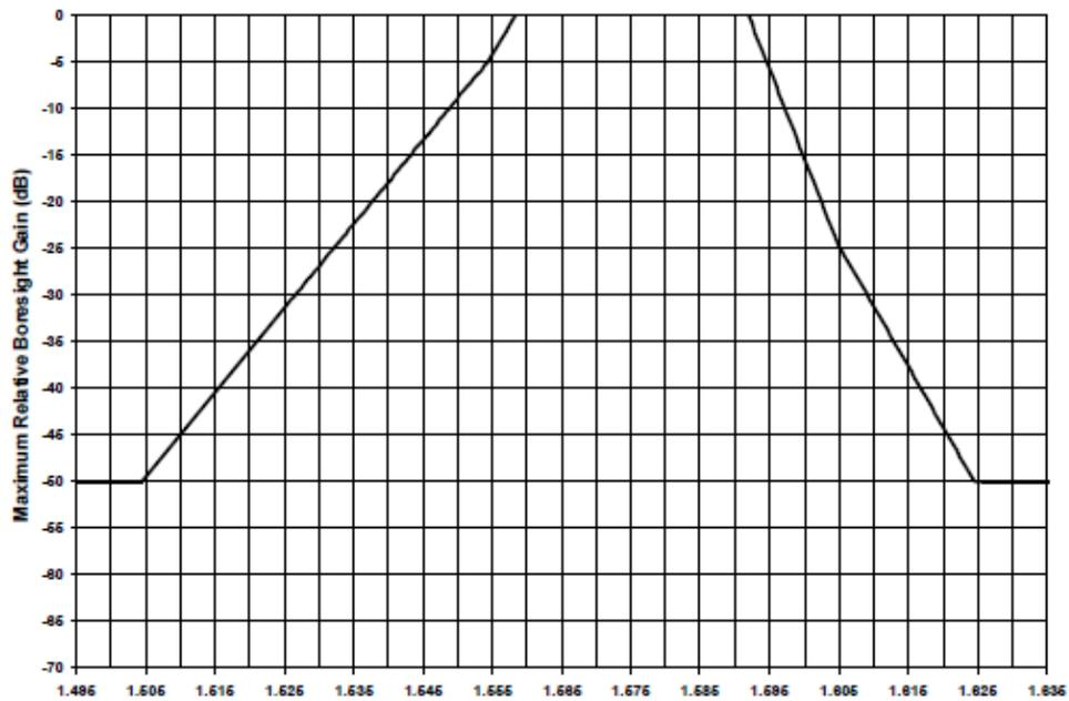
Figure 13: RTCA-DO-301 RF filter in graphical form
