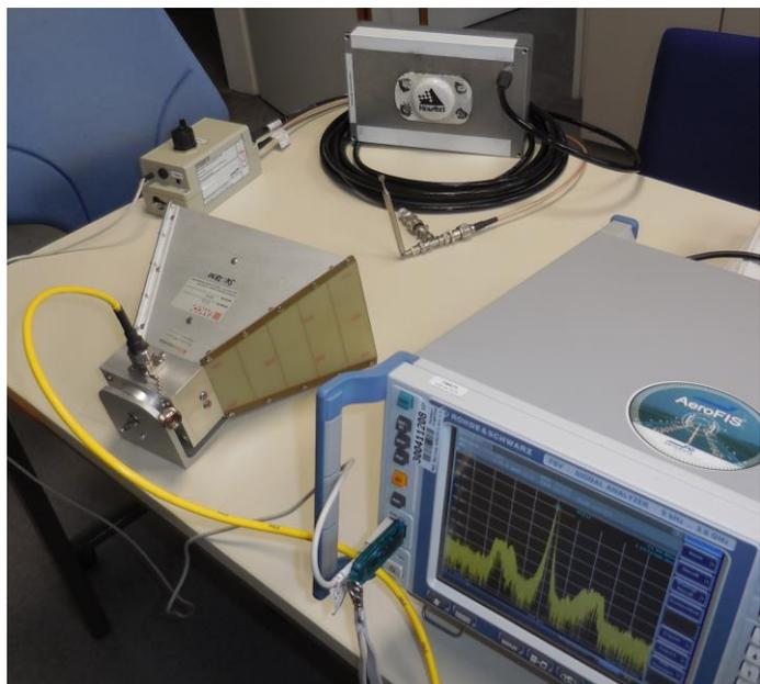
Figure 10: Test set up to produce oscillations by an open feed-back-loop
