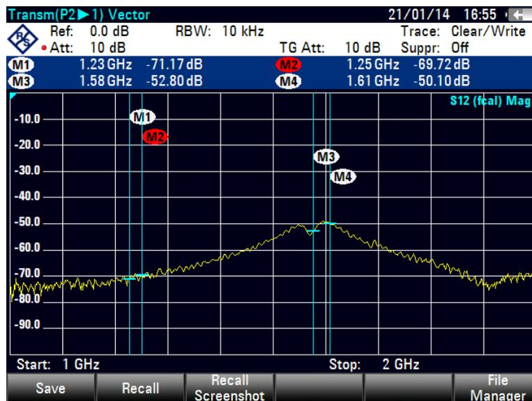
Figure 5: Passive Antenna
