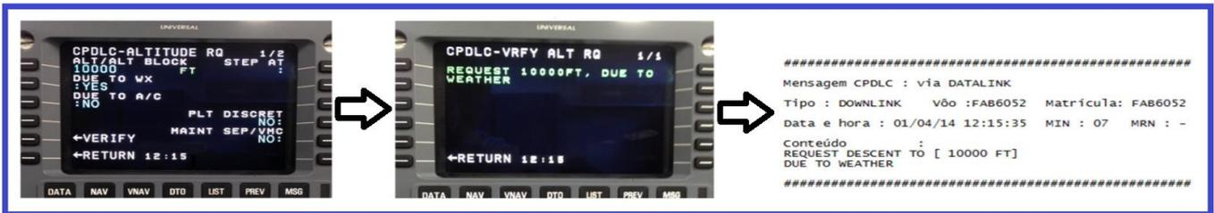
Data Flow for, request, approval, and logging of aviation data link traffic
