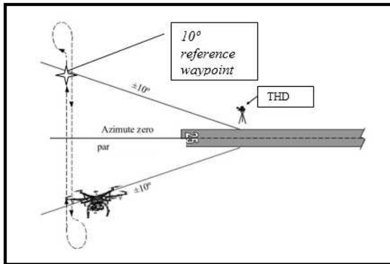
Fig. 7 – RPAS Angular Coverage in the Visual Navaid Flight Inspection Concept.
