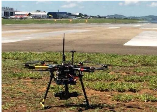
Fig. 5 – RPA used in third test of Visual Navaid RPAS flight inspection. (Source: GEIV)
