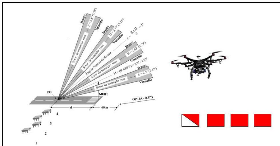
Fig. 6 – RPAS Transition Angle Inspection Concept.
