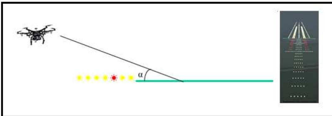
Fig. 9 - RPAS Operation, Intensity and Brightness of Lights of the ALS Flight Inspection Concept.
