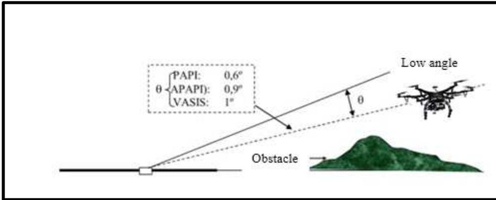
Fig. 8 - RPAS Obstacle Clearance in the Visual Navaid Flight Inspection Concept.
