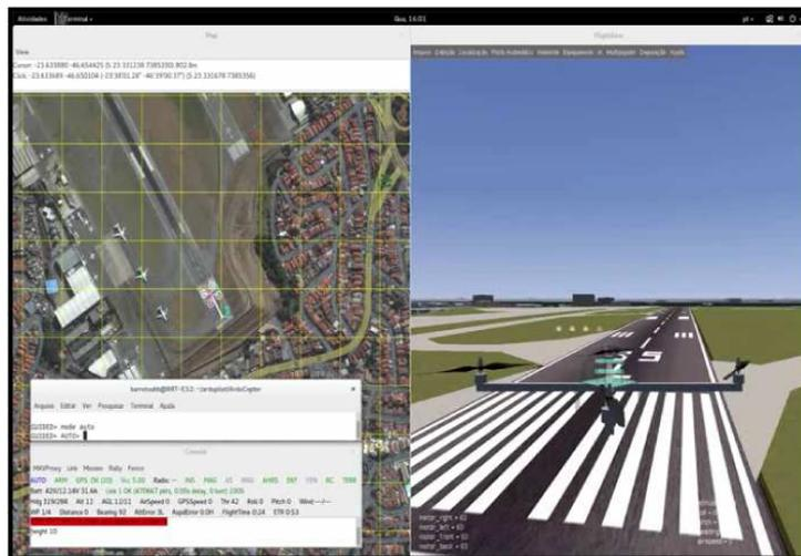
Fig. 4 – Simulated environment for RPAS flight inspection of Visual Navaid (Source: ICEA)
