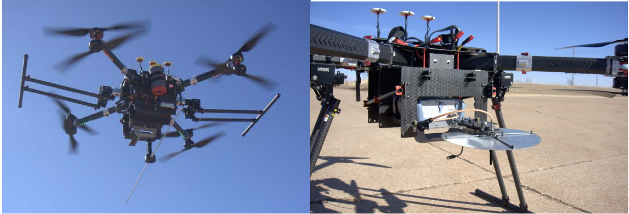
Figure 10: UAS with VOR/LOC measurement dipole mounted beneath (left) and vertical monopole (right)
