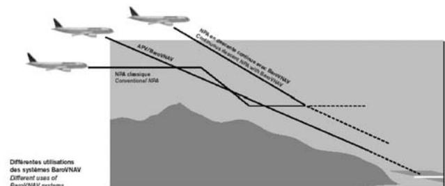
Figure 5. Different uses of BaroVNAV systems.
