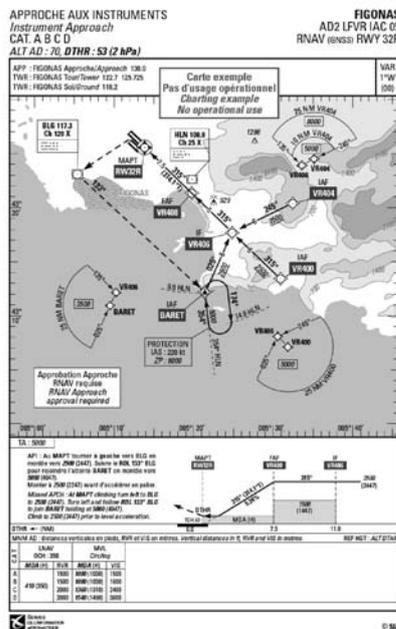
Figure 3. Typical RNAV approach chart for ABAS GNSS approaches showing minima for NPA/GPS (LNAV)
