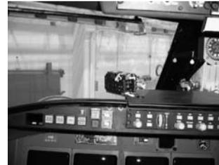
(Figure 5) (Installed Sony Cameras)
