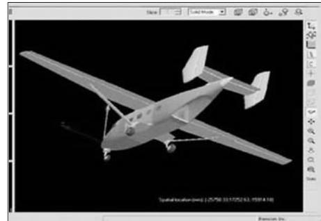
After importing the M28 geometry into XFDTD, it became clear the CAD file supplied did not describe the complete aircraft. The model lacked a rear hatch and the engines and propellers were absent. Using XFDTD geometric primitives and Boolean operations, the missing components were added to the aircraft.
