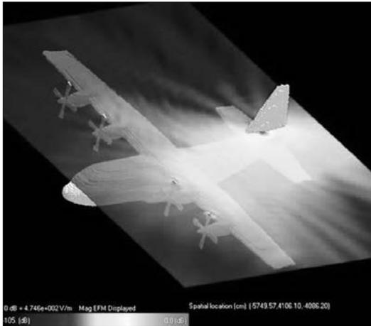
The figures below show the modeled azimuth plane radiation pattern for the C-130. Notice the very uniform coverage for the Phi (horizontal) polarization, which is of primary importance for flight inspection operations. This is an expected result given the symmetry of the aircraft empennage.
