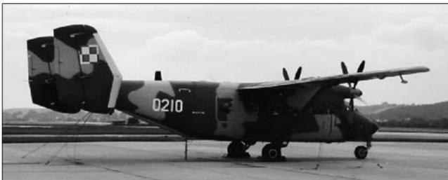
The dual-vertical stabilizers of the M-28 presented an unusual configuration for a flight inspection aircraft, and the effect of this type of empennage on VHF navigation antenna performance was unknown.
