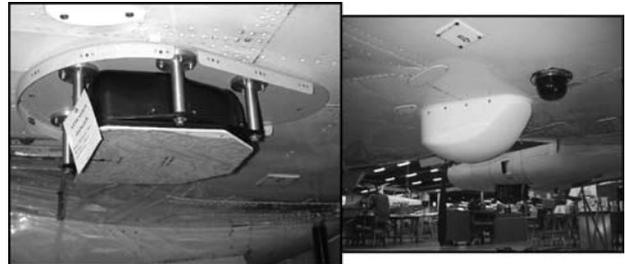
Figure 4 : The direction finder antenna fitted under the aircraft
