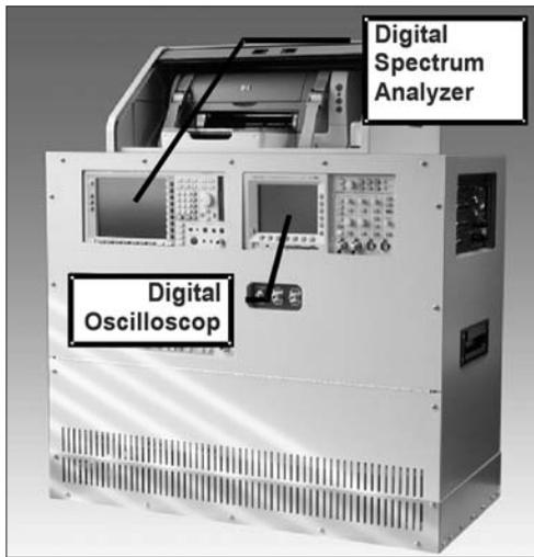
**Figure 3: Console with FSA and Oscilloscope**
