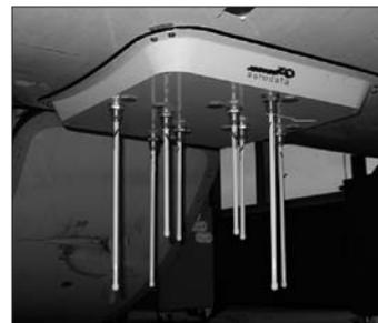
**Figure 8: DF VHF/UHF Antenna Array**
