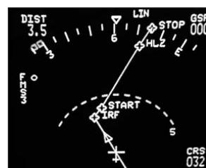
Figure 14: AFIS guidance on cockpit EFIS
