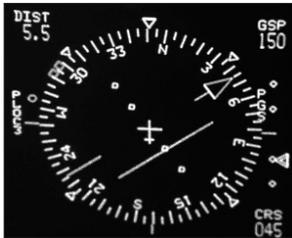
**Figure 15: AFIS controlled EFIS indicators**
