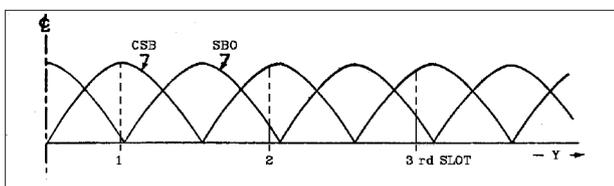
Figure 25. SBO and CSB Standing Waves Modes in the Middle of the Antenna
