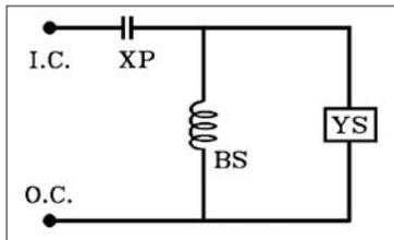
Figure 22. Equivalent Circuit of Slot Assembly
