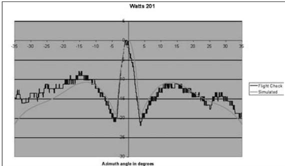
Figure 36. Total RF Level (Course and Clearance). Simulated (Pink) and Measured by the Flight Check (Blue)
