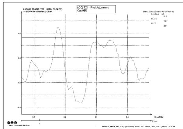
Figure 6. Course Structure on 16th September 2004 (Zoom in of Short Final Segment)
