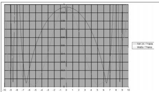
Figure 8. Bend Potential Reduction Referenced to the Thales 20+5 Versus Azimuth Angle (Normarc 3525 / Thales 20+5 in Blue, Watts 201 / Thales 20+5 in Pink)
