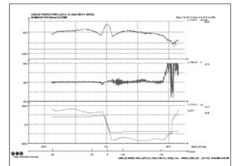
Figure 47. Flight Check of the Azimuth Transverse Structure in March 2006
