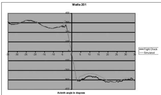
Figure 37. DDM Azimuth Profiles: Simulated (Pink) and Measured by the Flight Check (Blue)
