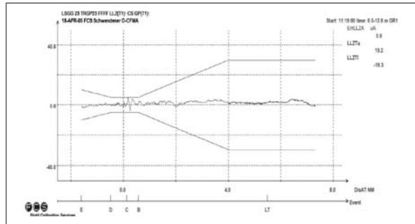
**Figure 14. Flight Check Results of the Normarc 3525 (Course and Clearance): Course Structure**
