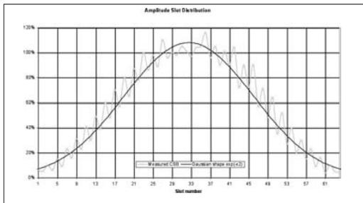
Figure 30. Gaussian Voltage Distribution for CSB (Theoretical and Measured)
