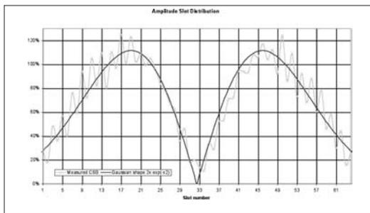
Figure 31. Gaussian Derivative Voltage Distribution for SBO (Theoretical and Measured)
