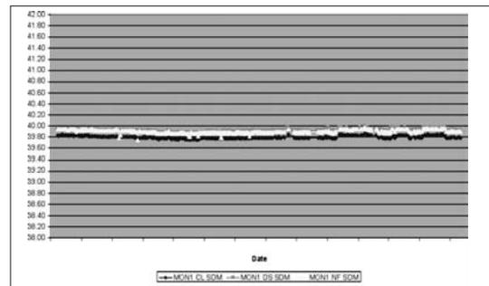
Figure 40. Monitor Stability Data between April 2005 and April 2006: SDM of the Course Integral Monitor Centerline (CL) in Blue, Displacement Sensitivity (DS) in Pink and the Nearfield Monitor (NF) in Yellow
