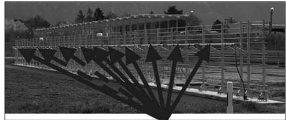
Figure 18. The Course Antenna Comprised of 16 Slotted Cable Sections
