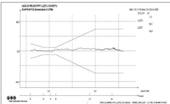
**Figure 12. Flight Check Results of the Combined System Watts 201 + Normarc 3525: Course Structure**
