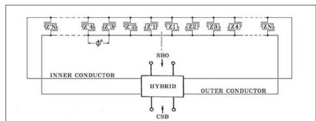
Figure 21. Equivalent Circuit of the Antenna
