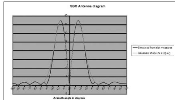
Figure 33. Gaussian Antenna Diagram for SBO. Theoretical (Pink) and Computed from Slot Measurements (Blue)
