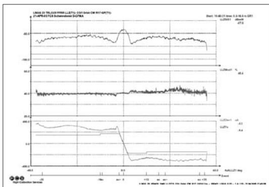
**Figure 13. Flight Check Results of the Combined System Watts 201 + Normarc 3525: Azimuth Transverse Structure (Field Strength in Green, SDM in Blue, DDM in Pink)**
