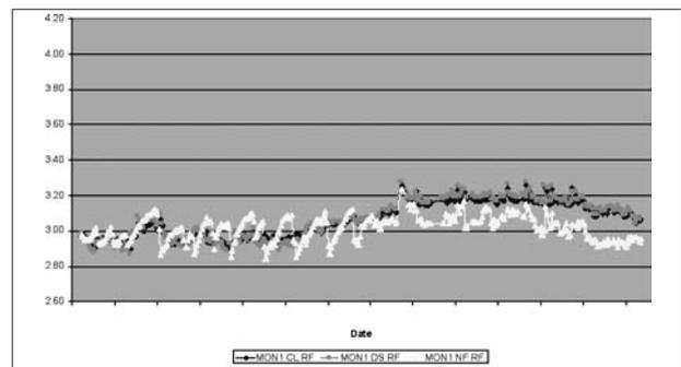
Figure 41. Monitor Stability Data between April 2005 and April 2006: RF Level of the Course Integral Monitor Centerline (CL) in Blue, Displacement Sensitivity (DS) in Pink and the Nearfield Monitor (NF) in Yellow
