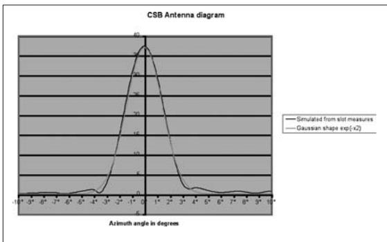
Figure 32. Gaussian Antenna Diagram for CSB. Theoretical (Pink) and Computed from Slot Measurements (Blue)
