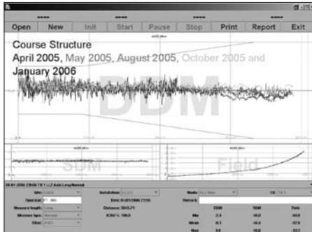
Figure 42. Ground Measurements of the Course Structure in April, May, August, October 2005 and January 2006
