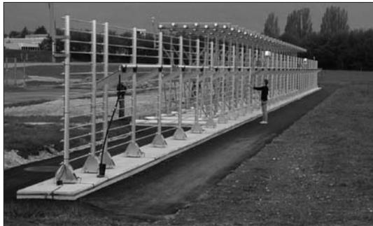
**Figure 11. Combined System Watts 201 + Normarc 3525 During Slot Measurements**
