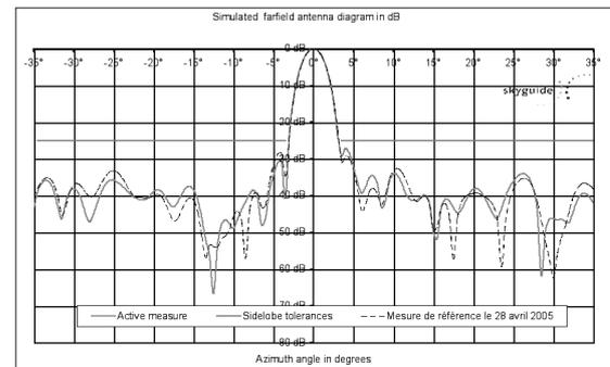
Figure 35. CSB Antenna Diagrams: Simulated from Slot Measurements (Pink)
