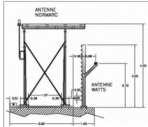
Figure 9. Vertical Layout of the Combined System: Watts 201 for the Course Signal and Normarc 3525 for the Clearance Signal
