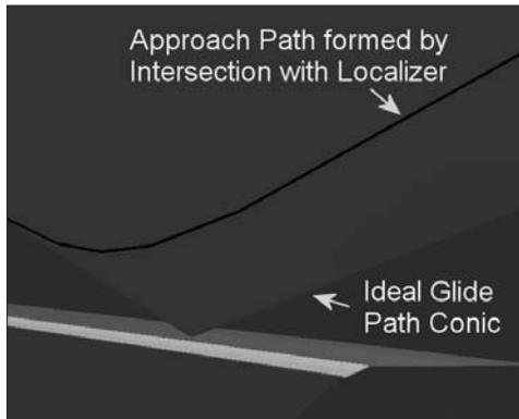
The previous figure does not show the effects of the lateral terrain slope. The lateral slope changes the geometry of the ideal conic and its intersection with the localizer.
