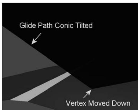
These two effects work in opposing directions. The tilting of the conic increases the height of the approach path, but the vertical moving down of the vertex decreases the height of the approach path. It has been shown that for lateral terrain slopes of up to 5%, these two opposing effects essentially cancel<sup>1,2</sup>.
