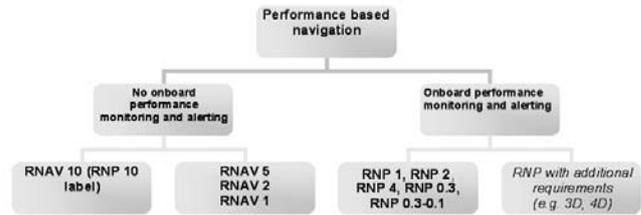
**Figure 2. Performance based navigation concept. In bold, navigation specifications that already have an operational requirement or that are in development. Navigation specification in *italic* are examples of potential expansion after assessment of performance objective.**
