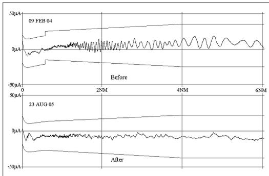
Figure 4. Typical glide path records before and after antenna modification
