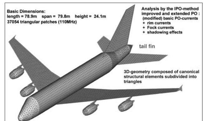
Fig. 2: A380 numerical 3D-model, scattering object.
