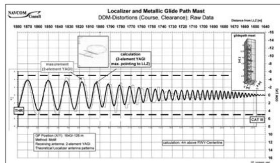
Fig. 9: DDM distortions of a lattice type glideslope mast (raw data); system simulations by using MoM compared to ground measurements.
