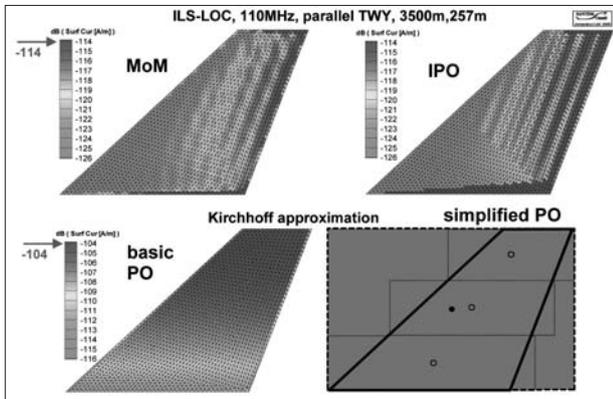
Fig. 10: Currents induced on a tail/fin like metal plate; different numerical methods: rigorous MoM, improved physical optics IPO, basic PO (uses Kirchhoff but for small patches), simplified PO (assumes constant current on the representing rectangle).
