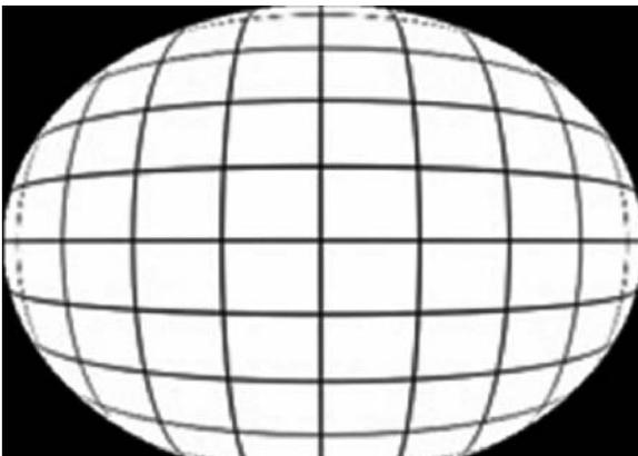
Figure 7 - Barrel distortion
