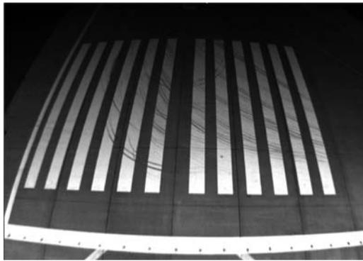
A wider field of view lens will give higher chance of capturing the region of interest even with severe aircraft roll, pitch and heading offsets.
