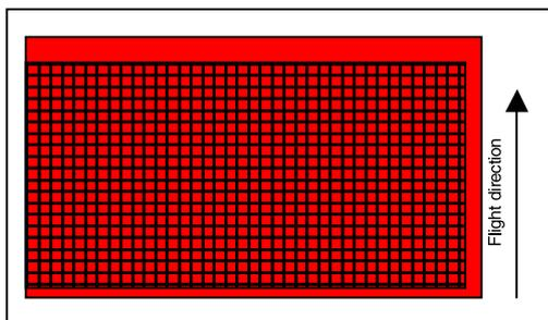
Figure 5 - Area scan covering entire area of interest in one instance
