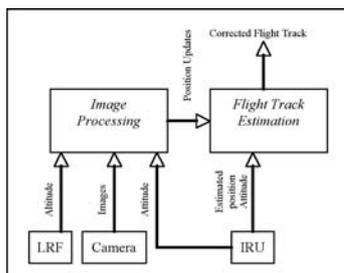
**Figure 1 - Typical camera / LRF / IRU coupled system**
