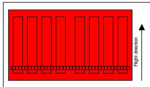
**Figure 2 - Line scan camera covers one pixel line at a given time**
