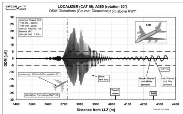
**Figure 7. Flight Measurements at 15 Meters, Varying Filter Characteristics, Proper Sampling**
