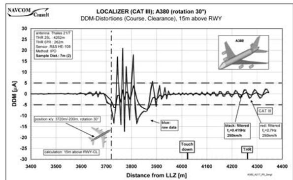
**Figure 8. Flight Measurements at 15 Meters, Varying Filter Characteristics, Insufficient Sampling Rate**
