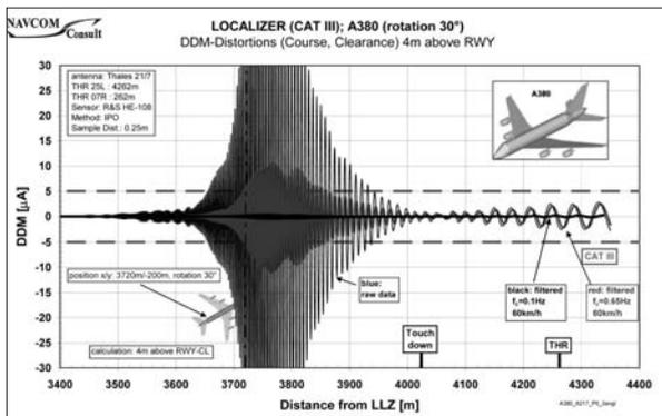
**Figure 6. Ground Measurements at 4 Meters, Varying Filter Characteristics, Proper Sampling**
