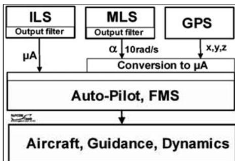
Figure 4. Multi-Mode Receiver feeding Avionics and Aircraft Systems
