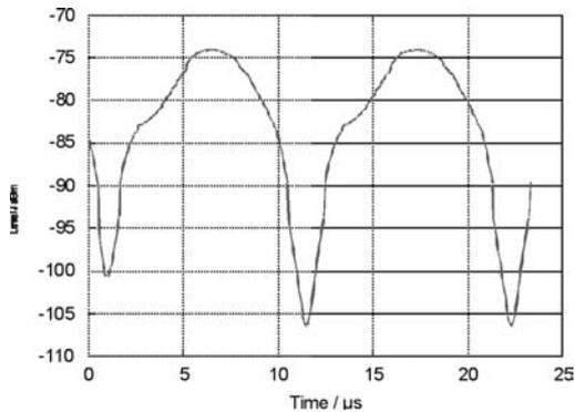
**Figure 4: Distorted DME Pulse Pair Visualized with SISMOS**
