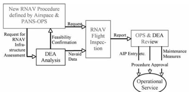
Figure 2: Signal-in-Space Assessment Process for RNAV Procedures
