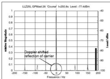
Figure 5: LLZ25L course signal spectrum with reflecting GP mast 26
