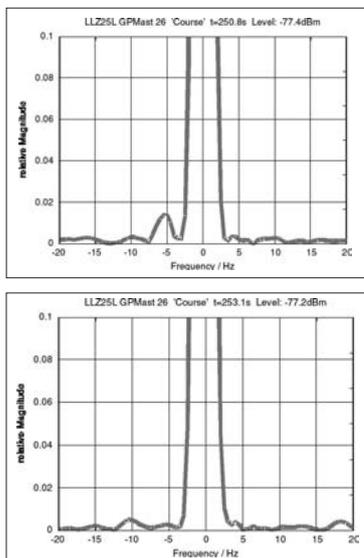
Figure 6: Spectral movement of the reflecting GP mast 26 (enlarged)
