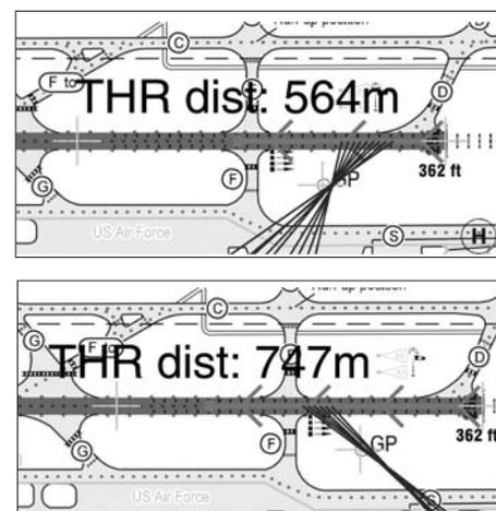
**Figure 3: Locating the GP mast 25L as a punctual scatterer from the front and from behind**
