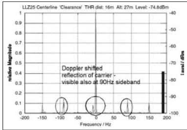
Figure 13: Clearance spectrum close to THR
