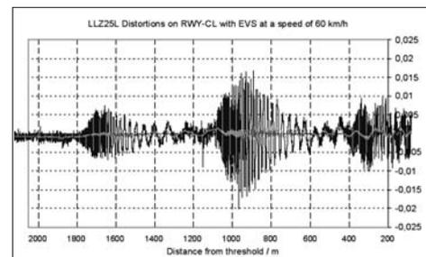
**Figure 2: Corresponding DDM record of ground vehicle equipped with EVS200 (blue, big amplitude indicates raw data while the small red indicates filtered data)**
