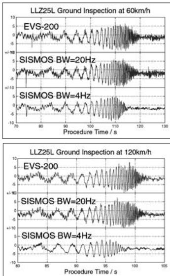
Figure 9: DDM of vehicle ground inspection at different speed and 90/150Hz sideband filters affected by reflection of GP mast 26
