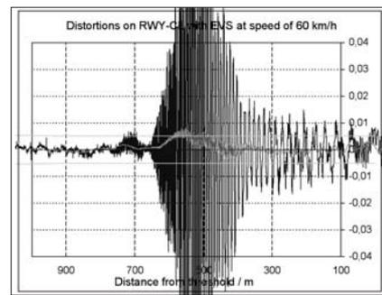
Figure 14.1: Distortion measured on RWY centreline with a speed of 60 km/h (Receiver EVS 200), with raw data in blue (big amplitudes) and filtered data in red (small amplitudes).
