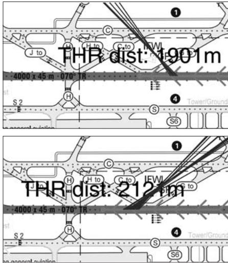
Figure 4: Locating the GP mast 26 of HALS/DTOP
