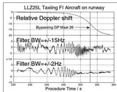
Figure 8: DDM of aircraft on ground with different 90/150Hz sideband filters affected by reflection of GP mast 26
