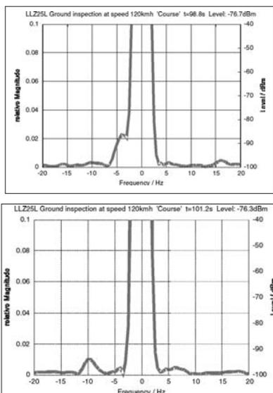
Figure 10: Spectral movement of the reflecting GP mast 26 during vehicle ground inspection
