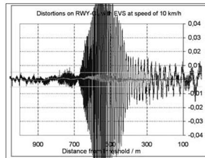
Figure 14.2: Distortion measured on RWY centreline with a speed of 10 km/h (Receiver EVS 200), with raw data in blue (big amplitudes) and filtered data in red (small amplitudes)
