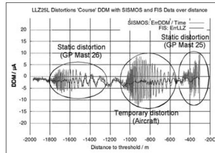
**Figure 1: DDM of aircraft during landing with static and artificial distortions (EDDF LLZ25L)**
