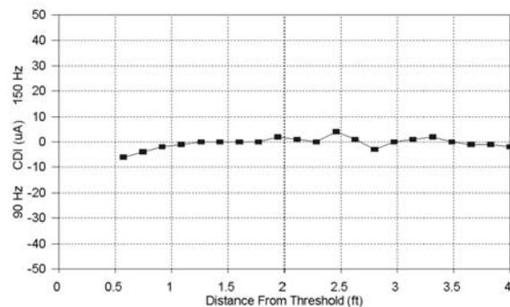
Figure 5: Glide Path Performance before Upper Antenna was Canted
