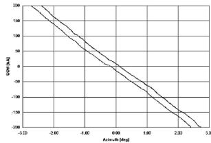
**Picture 9 The difference between clockwise and counter clockwise flight - effect of receiver’s delay**
