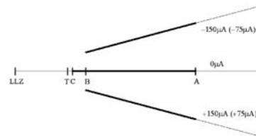
Picture 2 Approach method of the course width measurement
