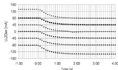
**Picture 8 Receiver reaction on step changes of the DDM**
