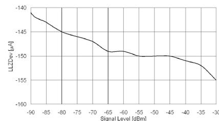
**Picture 7 Localiser Deviation after correction using of SDM reading for -15.5% DDM**
