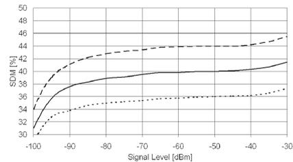
**Picture 6 Sum of Modulations reading versus input signal level**
