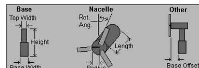
Figure 3. Wind turbine parameters for simulation
