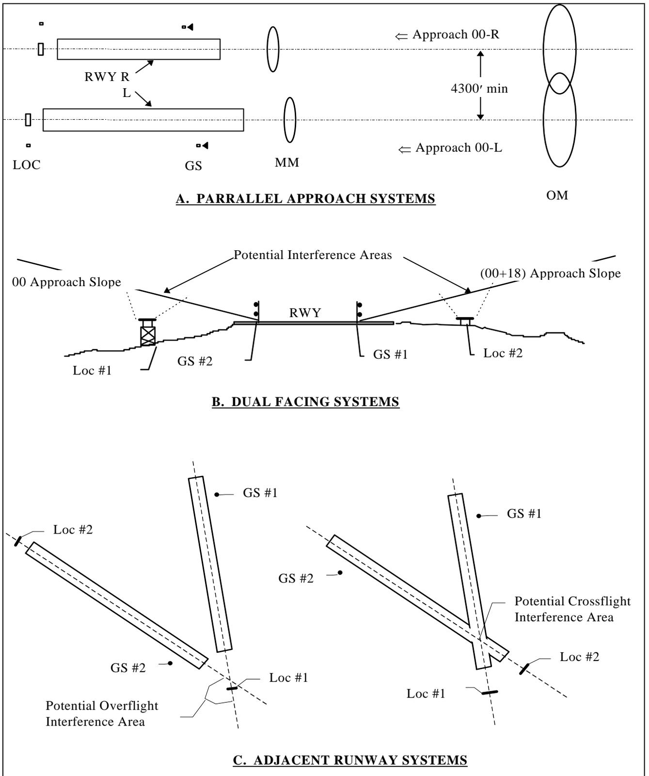
Figure 1. Multiple ILS Configurations
