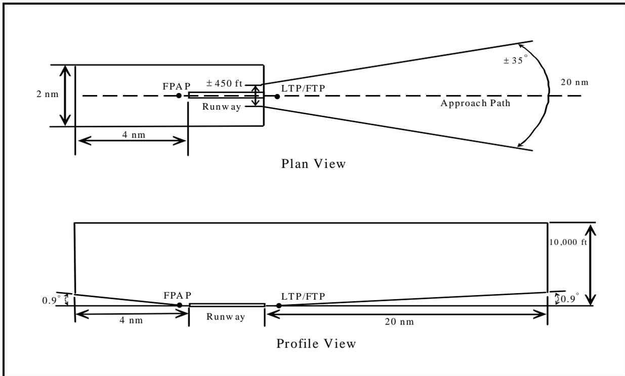
**Figure 3. LAAS Approach Coverage Requirements.**
