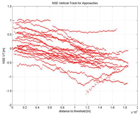
**Figure 6. NSE vertical track versus distance to threshold**
