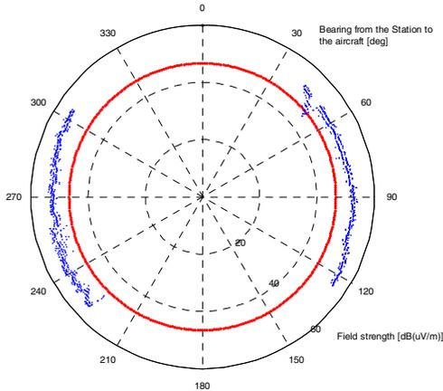
**Figure 8. Field strength of +/-35°-Arc**
