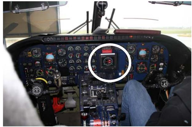
**Figure 2. Cockpit of Research Aircraft with experimental CDTI**
