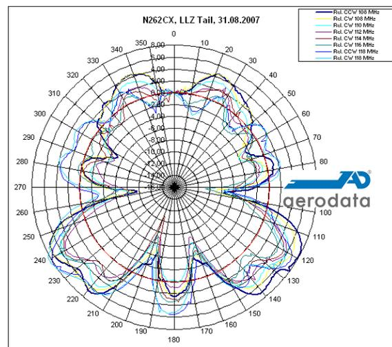
**Figure 9. Antenna calibration diagram**
