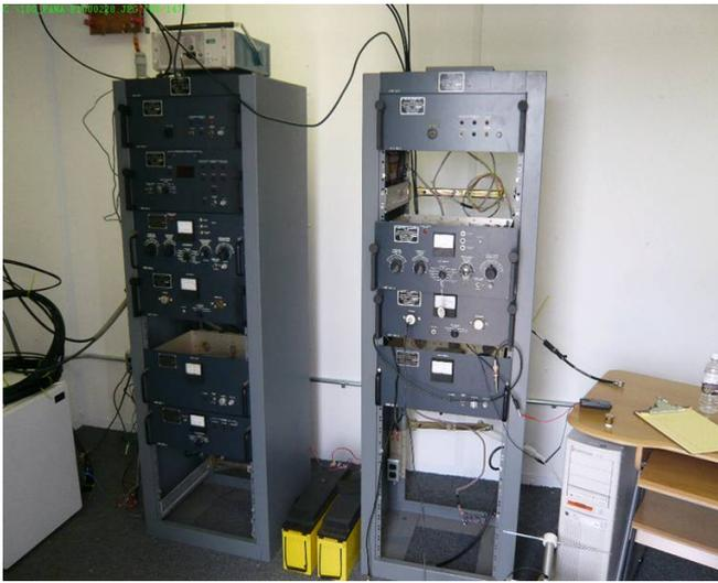
Figure 2. Picture Showing the Glide Slope Transmitting Equipment Used to Generate RF Signals for the Steep Angles. Transmitter on the Right is for 5.5 Degrees and on the Left for 6.65 and 8.65 Degrees.
