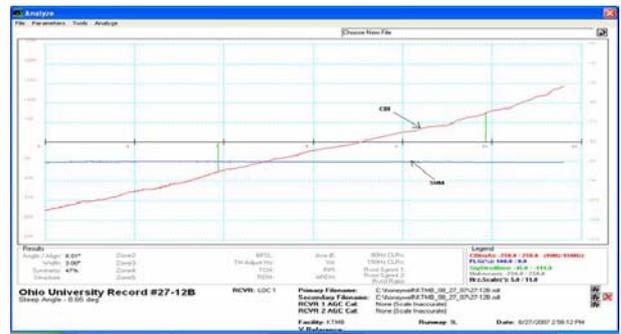
Figure 7. Measured Glide-Slope Guidance Performance (8.65 Degrees). [8/27/07]
