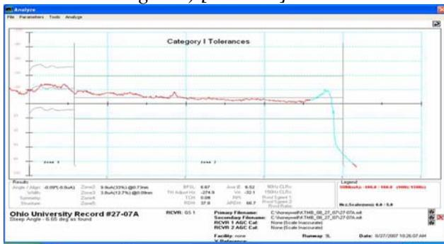
Figure 10. Glide-Slope Path Quality (Category I Tolerances) (Path Angle 6.65 Degrees).[8/27/07]
