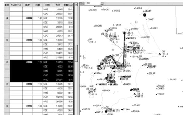
**Figure 8: Sample of DME list generated by JCAB Flight Inspection map tool**
