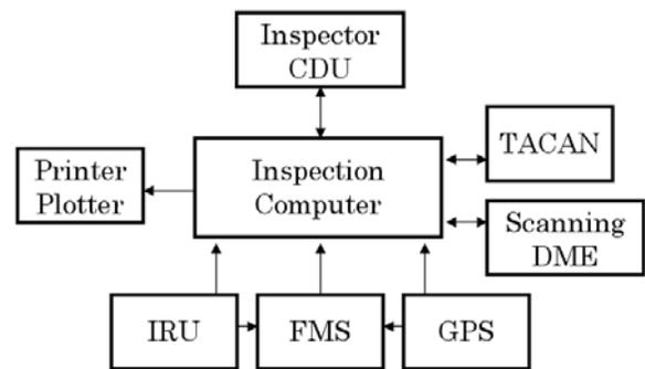
**Figure 6: Schematic diagram of the DME/DME RNAV Inspection system**
