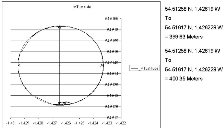
**Figure 2: Circle described by rotating GMPU over a fixed position**
