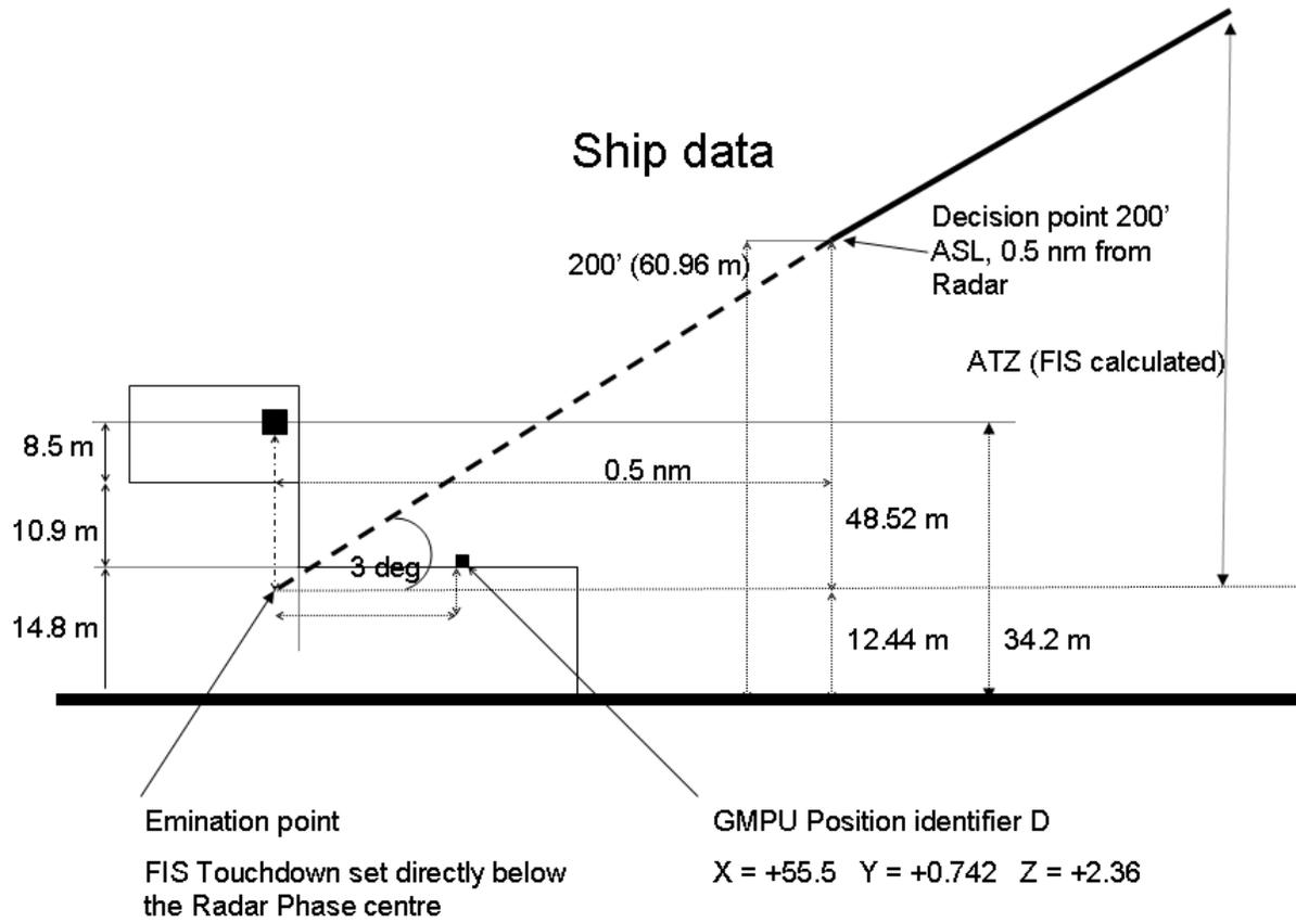
The PAR system is designed to bring an aircraft to a point 200' above the sea surface at 0.5NM from the Radar Antenna.
