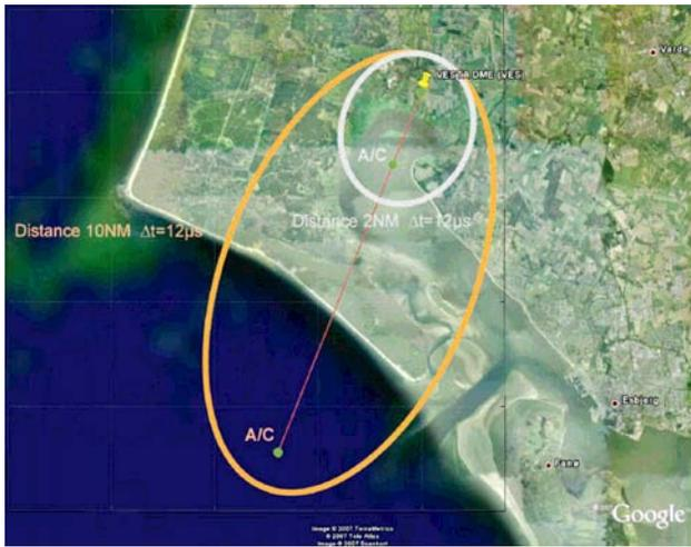
**Figure 7: X-Channel Spacing Critical Multipath Ellipses**
