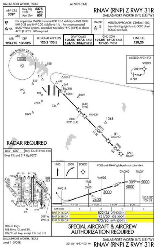
**Figure 8 Approach Plate for RNAV Z RWY 31R**
