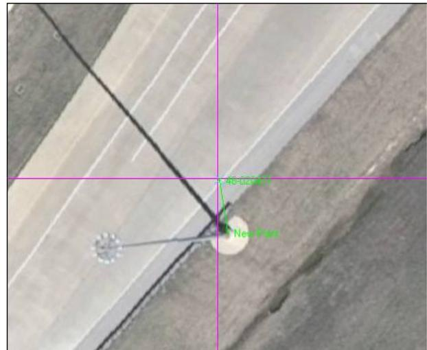
**Figure 5 SmarTopo view of light pole obstacle using aerial survey imagery.**
