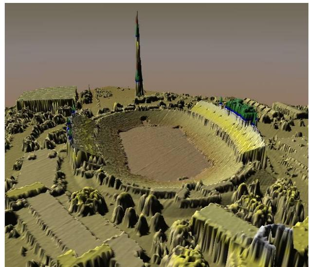
**Figure 6 LiDAR image of the Cotton Bowl.**
