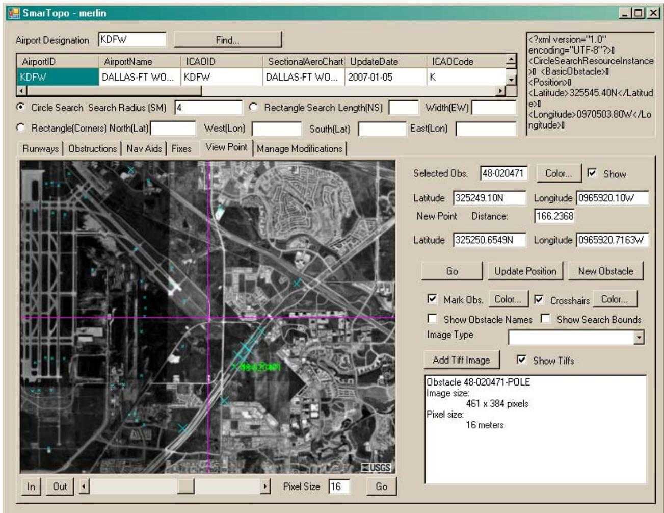
Not all of these light poles were entered in the AirNav database, but those that were had a vertical accuracy of 76 meters horizontally and 15 meters vertically. Because their position was not precisely known, the approach minima had to be increased accordingly. It was thought that this would be a practical test for the real-world utility of SmarTopo. Could SmarTopo be used to lower the approach minima for DFW RNP Z31R?
