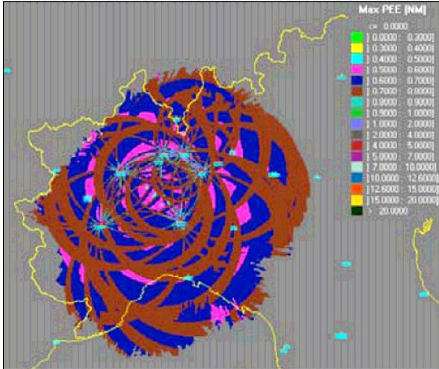
Figure 6 - Sample of DME positioning error estimate on an area
