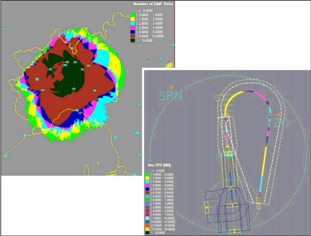
Figure 5 - Samples of DME pairs computation along procedures and areas
