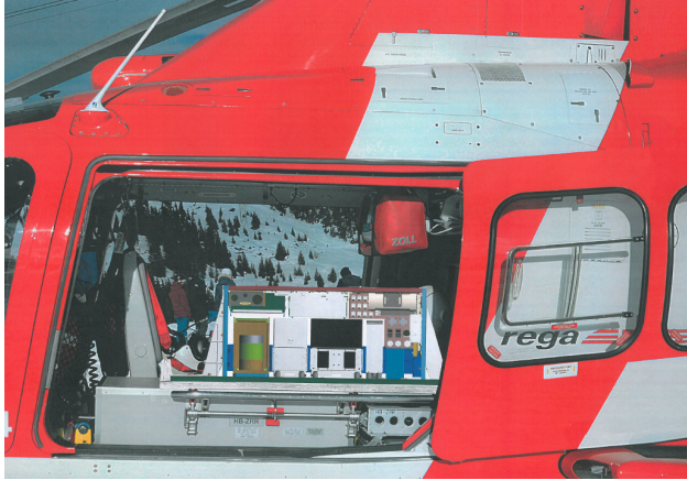
Figure 10. HeliFIS installed in AW109SP
