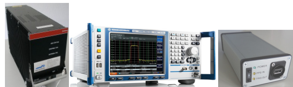
Figure: Collins GNLU-930, spectrum analyzer and UTC time synchronization box
