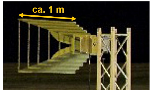
Figure 7: Double-Ridged Horn Antenna Mounted to a Mast
