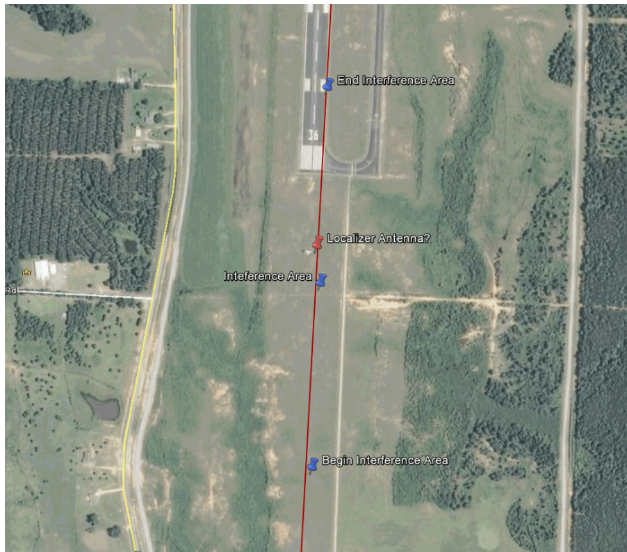
Figure 2. Close Up View of Interference Area
