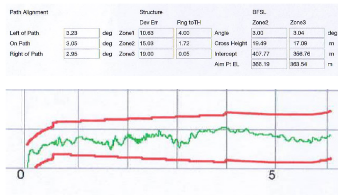
Figure 9. Results And Glide Path Deviation Error Curve Using 362.38m as Glide Path Reference Point Elevation
