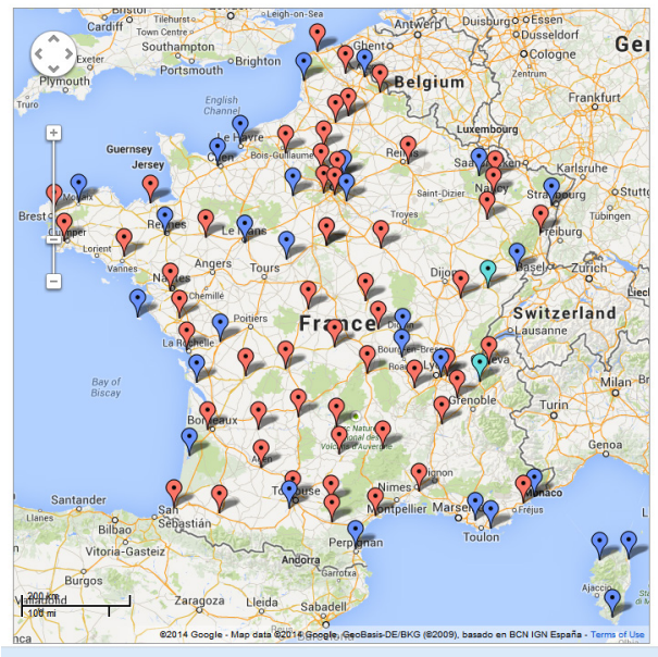
Figure 1 : Flight inspected RNAV(GNSS) Procedures on French mainland territory (As of 01/March/2014) (Red : LNAV+LPV, Blue : LNAV only, Clear Blue : Trials)
