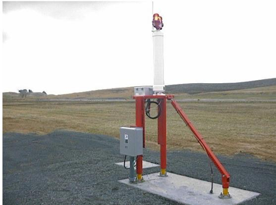
**Figure 12: The Calibration / Built In Test transmitter assembly is shown. It provides a 1090 MHz signal used to monitor the accuracy of the measurement subsystems. The assembly is 2 m tall, 40 Kgs (90 lbs) and mounted on frangible couplings.**
