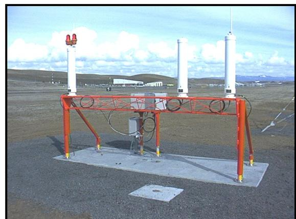
**Figure 10: The azimuth measurement assembly is shown with three antennas. Each antenna is vertically polarized with 6 receive elements. Main lobe peak is +3 degrees above the horizon. The assembly is 2 m tall, 105 Kgs (230 lbs) and mounted on frangible couplings.**
