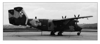
The dual-vertical stabilizers of the M-28 presented an unusual configuration for a flight inspection aircraft, and the effect of this type of empennage on VHF navigation antenna performance was unknown.
