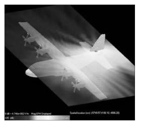
The figures below show the modeled azimuth plane radiation pattern for the C-130. Notice the very uniform coverage for the Phi (horizontal) polarization, which is of primary importance for flight inspection operations. This is an ex-pected result given the symmetry of the aircraft empennage.
