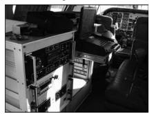
Figure 8 : Interference search bench installed on board the F-ASFA
