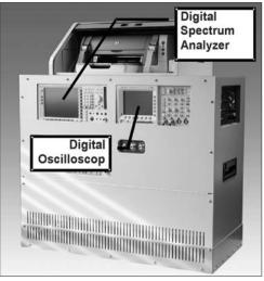
Figure 3: Console with FSA and Oscilloscope
