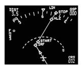
Figure 14: AFIS guidance on cockpit EFIS
