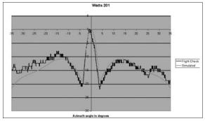
Figure 36. Total RF Level (Course and Clearance). Simulated (Pink) and Measured by the Flight Check (Blue)
