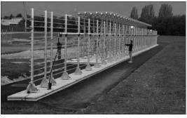
Figure 11. Combined System Watts 201 + Normarc 3525 During Slot Measurements
