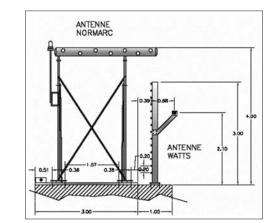
Figure 9. Vertical Layout of the Combined System: Watts 201 for the Course Signal and Normarc 3525 for the Clearance Signal
