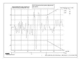
Figure 5. Course Structure on 15th September 2004 (Zoom in of Short Final Segment)
