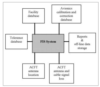
Figure 1 - Typical data integrity elements
