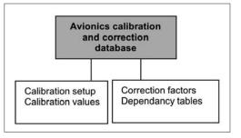
As with the other data integrity issues, the organization should have a way of quality assuring the calibration routines, and keep track of all information relevant to the calibration. This includes also such information as calibration date of signal generators etc.
