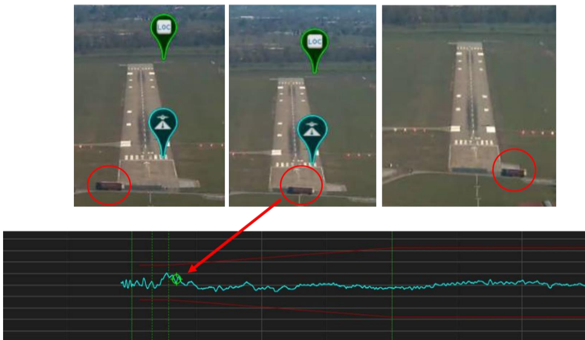
Fig. 10: Correlation of Video and Data Anomaly (Source: [1]). Moving truck vs. LOC deviation error
