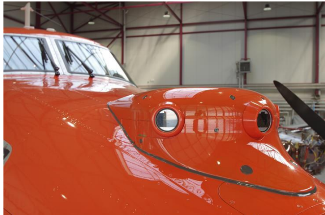
Fig. 2: Three Cameras mounted on Aircraft Nose (Source: [1])
