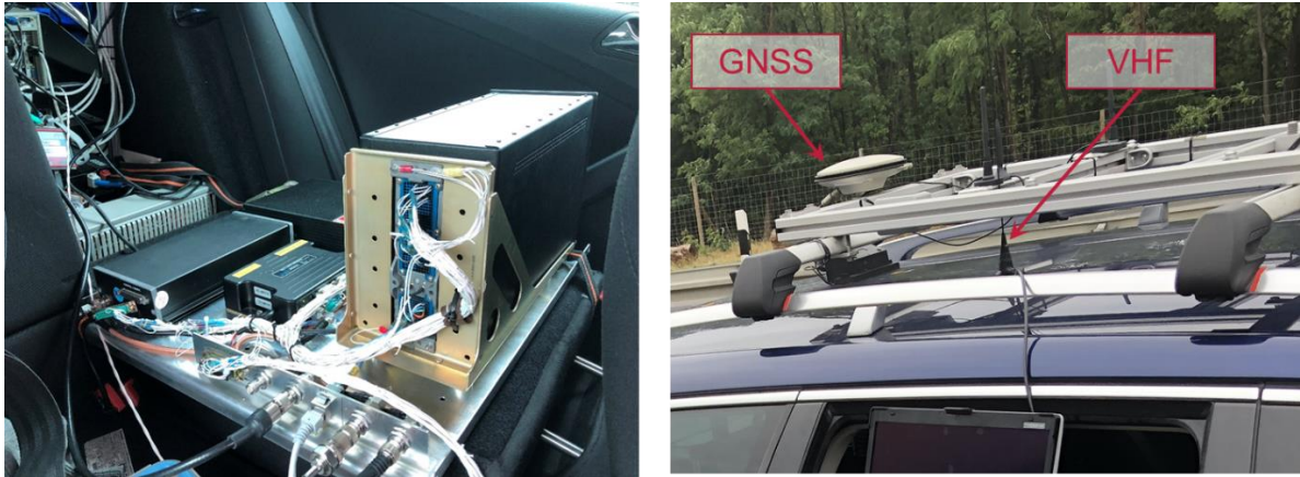
Figure 3: Integration of the GBAS FIS demonstrator into the TU Braunschweig research car
