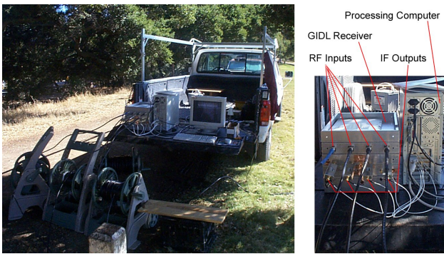
Figure 13: GIDL base station (GIDL receiver, processing computer, etc.) was located in the bed of HEPL truck during experiments at Lake Lagunita
