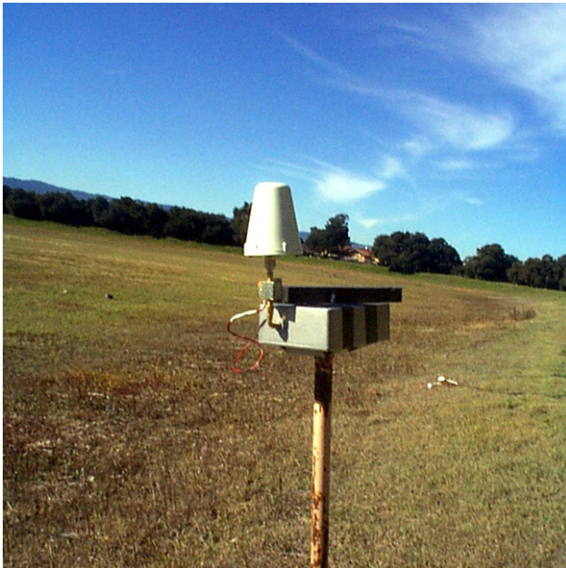
Figure 8: Experimental Jammer: -40 dBW/MHz white noise source
