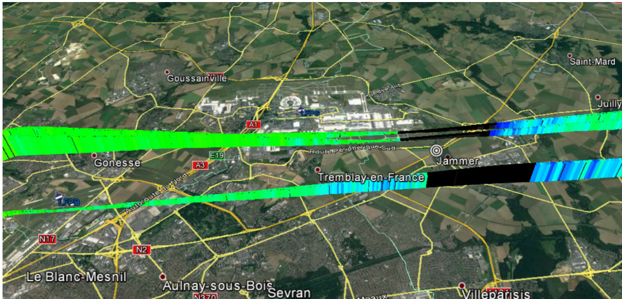
Fig 10 : Finals approaches on CDG and Le Bourget (Color function of the C/N0 parameter)
