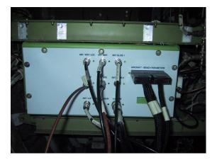
A special cable-set is connected before each calibration campaign between the bench and the junction panel. It is fixed on the aircraft's floor.
