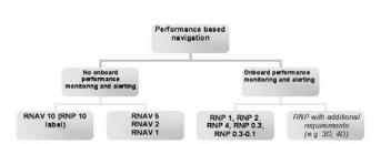
Figure 2. Performance based navigation concept. In bold, navigation specifications that already have an operational requirement or that are in development. Navigation specification in italic are examples of potential expansion after assessment of performance objective.
