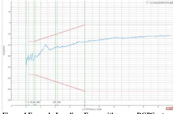
Figure 4 Example:Localizer Error with wrong DGPS setup
