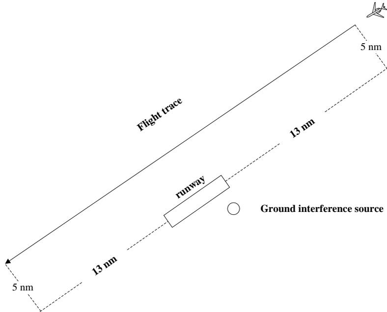
Figure4 Flight illustration for profile 2
