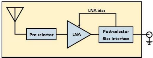
Block Diagram for active GNSS antenna
