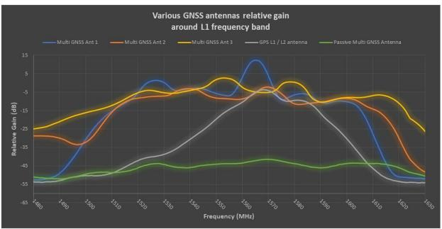
Various multi GNSS antennas frequency response around L1 frequency band
