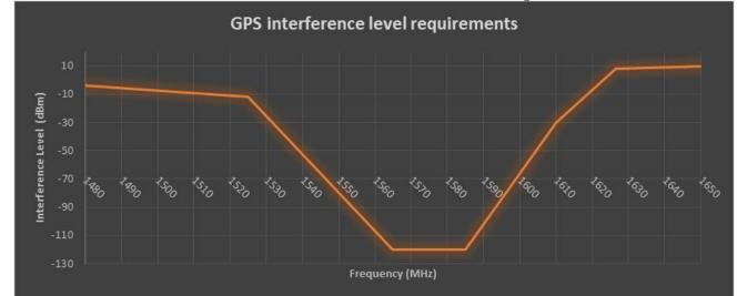
For CW interference in the GPS L1 band the receiver shall be able to handle the following levels:
