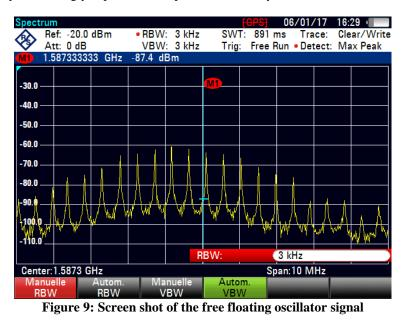
The free oscillating GPS antenna amplifier had an unstable center frequency of 1.5873 MHz, close to L1
