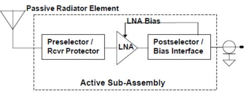
Figure 1: Typical Block diagram of an active GNSS antenna
