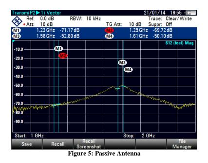
This passive antenna was designed for L1 only. Signal is approx. 30 dB lower compared to amplified antennas
