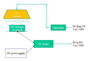
Figure 2: System Block diagram (simplified)
