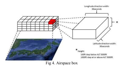
Airspace box size: 30 seconds  $\times$  30 seconds  $\times$  height \*
