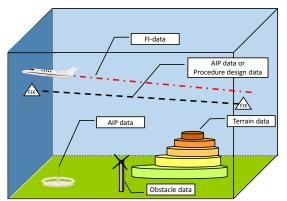
Fig 2. The data used for display in FIDM
