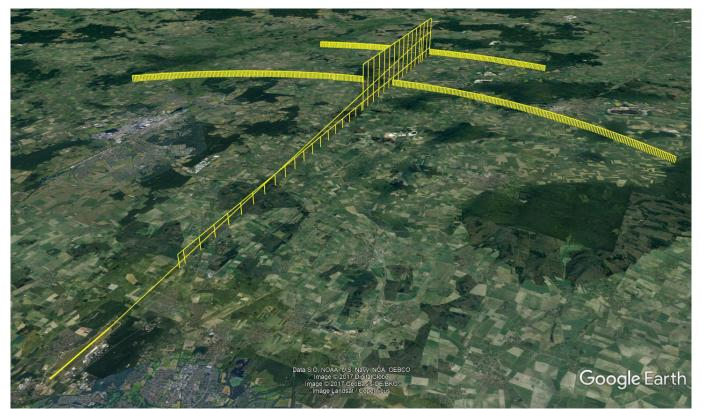
Figure 4: Exemplary flight inspection procedures for a GBAS approach to Braunschweig-Wolfsburg Airport EDVE (Source: 52° 18' 23.18" N and 10° 46' 53.27" E. GOOGLE EARTH, December 14, 2015. October 24, 2017.)
